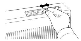
In order to stop operation, press the power switch to switch the unit off. The Air Blower Speed Lamp will go out.
