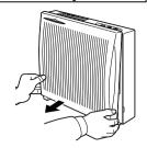
Remove the HEPA filter in the bag from the main unit.
