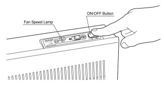
In order to switch the air blower speed, select "High" or "Low" with the Air Blower Speed Switch. The air blower speed lamp will also be activated.
