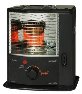
Spark ignition system (named "ponPa") ignites the wick by discharging electrical spark between two electrodes, by simply just giving the Main Knob a full turn to the right. This new uniquely designed spark ignition system is maintenance free and avoids any troubles of igniter coils, often found in conventional heaters.
