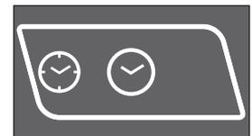
H: The TIMER indicator light indicates that the timer function has been switched on.
